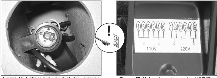
Figure 45. Light socket with dust plug removed (for 110V operation only).
